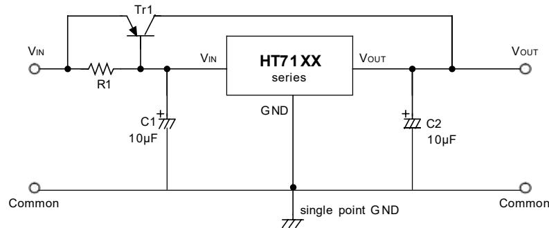
**Short-Circuit protection by  $Tr_1$**
