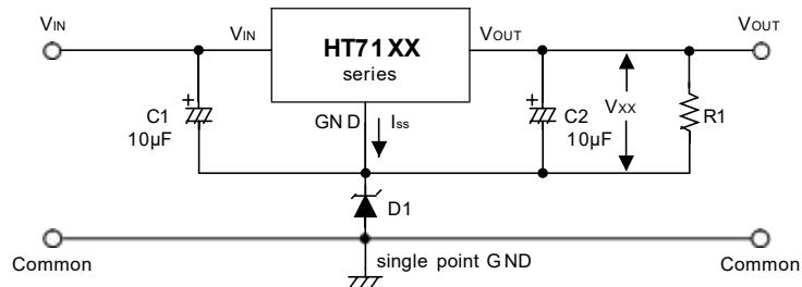
$$V_{OUT} = V_{XX} + V_{D1}$$
