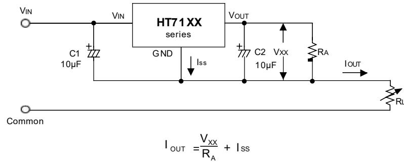
$$I_{OUT} = \frac{V_{XX}}{R_A} + I_{SS}$$
