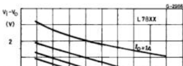
Figure 1: Dropout Voltage vs Junction Temperature
