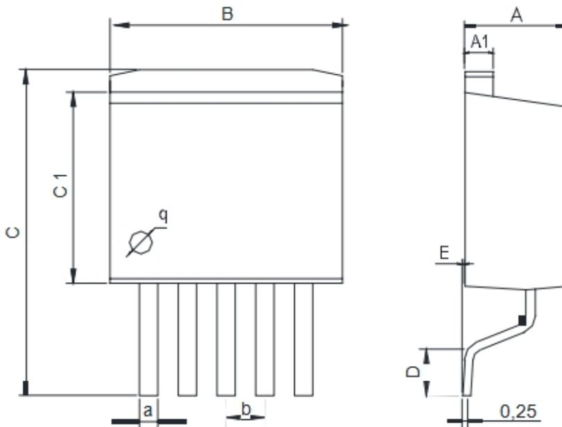
Dimensions In Millimeters(TO-263-5)
